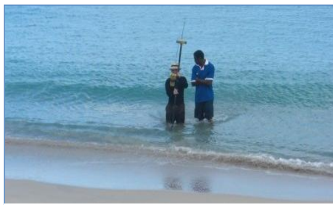
Figure 1: High Resolution Coastal Profile Surveying with GPS
