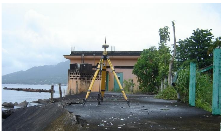
Figure 2: High Resolution Coastal Profile Surveying with GPS, Coconut Beach, Dominica.
