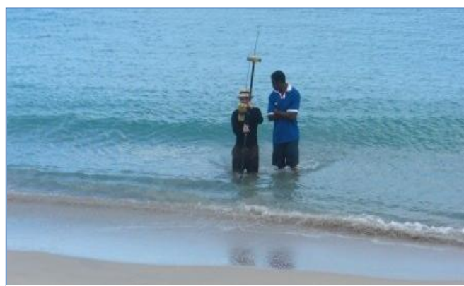
Figure 2: High Resolution Coastal Profile Surveying with GPS
