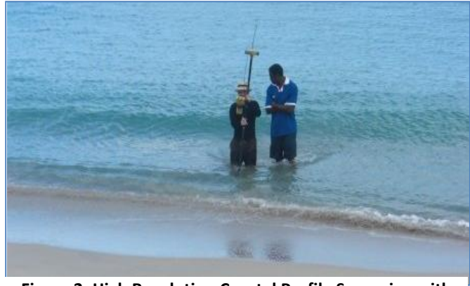
Figure 2: High Resolution Coastal Profile Surveying with GPS
