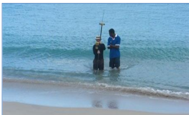
Figure 1: High Resolution Coastal Profile Surveying with GPS
