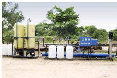
Figure 7: Small-scale reverse osmosis technology
