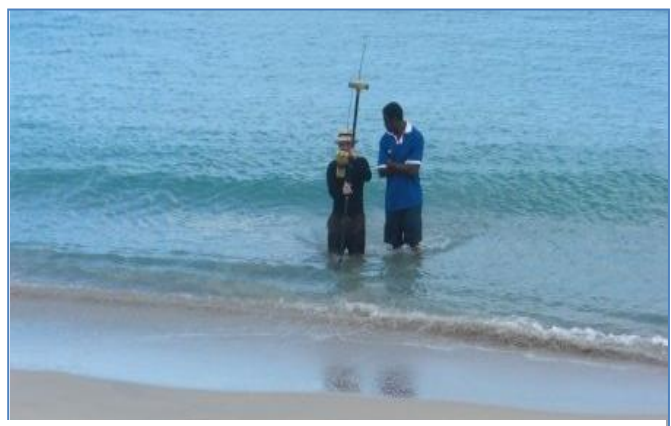
Figure 1: High Resolution Coastal Profile Surveying with GPS
